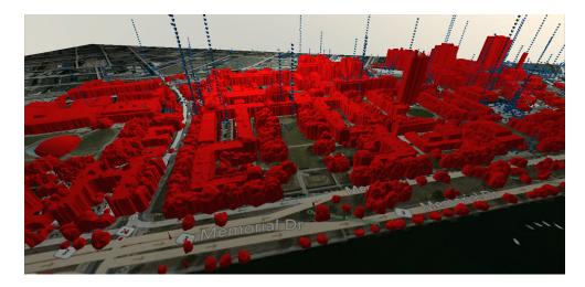
Figure 2-4: Rendition of MIT's campus imported FBX model View of imported MIT FBX model into the Unity3D engine as seen from game's free-form camera. These models are then superimposed on Google Maps textures matching the same scale and latitude, longitude bounds as the original LADAR data. Tweets are juxtaposed onto the scene based on provided mobile geo-tagged information.
