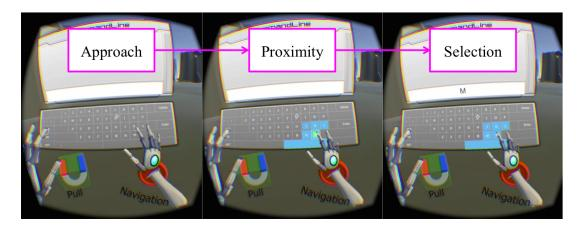
Figure 3-2: Leap Motion Interactable Keyboard
