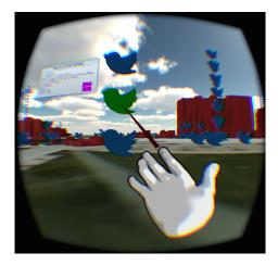
Figure 2-6: Debugging with the Leap Motion Controller Leap Motion hand controller allows the player's hands to be rendered in the simulated scene. Gestures and other inputs registered by the device can launch events and other commands intended by the user during analysis and gameplay.
