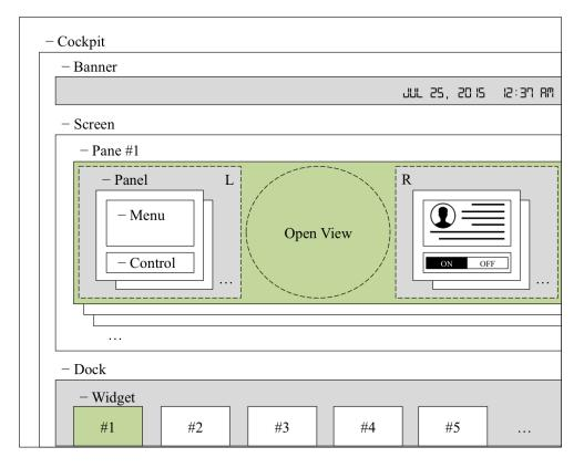
Figure 2-7: Schematic of VRLeapInterface Holodeck
