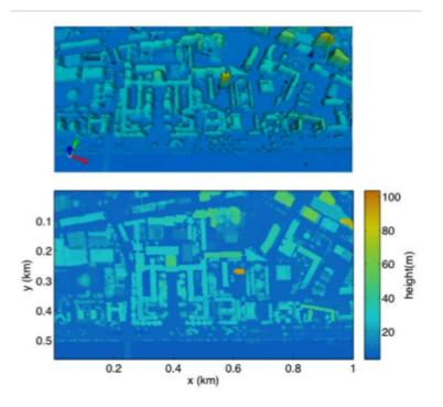
Figure 2-2: LADAR Image of Cambridge Height map of Massachusettes Institute of Technology generated from LADAR data in 2005. Final scan shows a 1m resolution image of approximately one square kilometer of Cambridge, MA.
