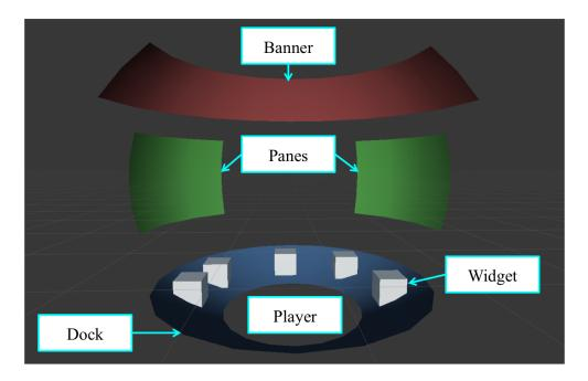
Figure 2-8: 3D mockup of VRLeapInterface Holodeck
